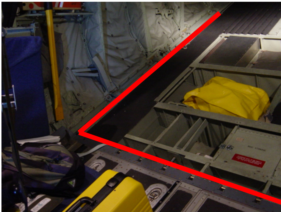
Figure 2. Starboard side, seam of rear cargo door, hot spots indicated in red.
